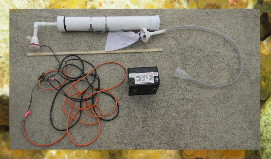
4" PVC...Approximately 28 inches in length. 34" suction hose with attached funnel. Inline mesh collection bag. 12v bilge pump.
